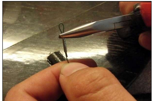
Figure 2.11 - Crimping tube cable
