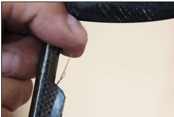
Figure 2.13 - The thread on the cable of the elevator
