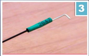
Slide heat shrink tube over the joint and drop CA inside the tube.
