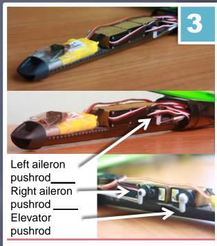
Glue servos with CA, but leave the battery mounted with tape.
