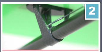
Mark the position of V-mount onto the tail boom. To eliminate the gap, remove the V-mount and wind thin thread around the boom.
