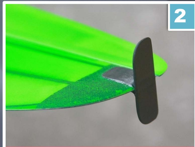
Install the peg on the wing tip and glue it with thin CA.
