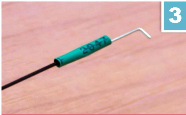
Slide heat shrink tube over the joint and drop CA inside the tube.
