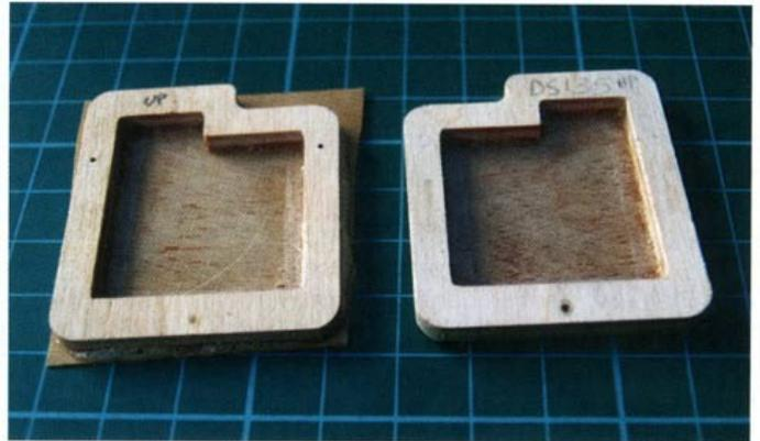
*Servo trays backed with thin ply before and after trimming. This allows positioning and installing without the fear of also gluing the servo permanently in place! Remember to clear the glue from the screw holes*
