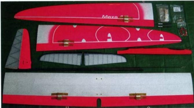
**Component spread.** Bags contain all the metal bits and bobs, wiring for Rx/wing connection and plastic servo hatch covers
