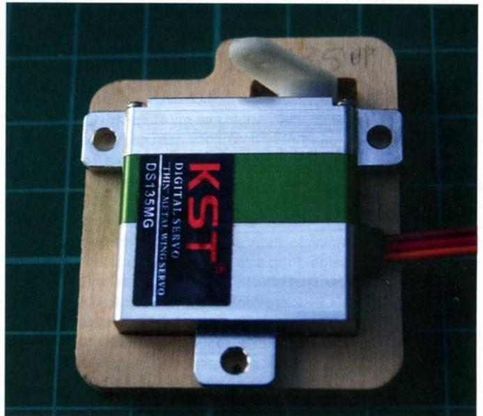
*KST 135 flap servo has hefty side mounting lugs for direct fixing to the ply frame. Metal gears seem very durable and the servo yields easily if the controls are touched when handling, which is an important feature to save damage*
