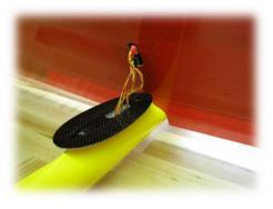
Figure 22: Connect the Wing wire harness
