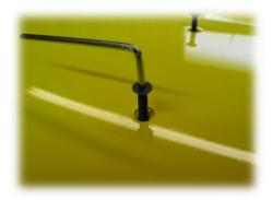
Figure 23: Attach the Wing to the Fuselage with 2 bolts
