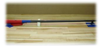
Figure 5: Shows fuselage and boom epoxied together, and secured to the table
