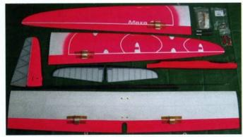
Component spread. Bags contain all the metal bits and bobs, wiring for Rx/wing connection and plastic servo hatch covers
