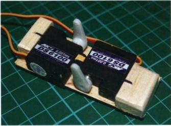
Elevator and rudder servos were fitted onto the balsa carrier and installed through the canopy before being bolted in place
