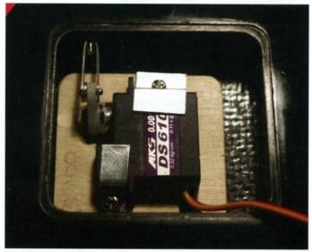
DS6100 installed in its frame with homemade clips to secure. Clear cover held in place with tape at this stage. Vladimir supplies a nice one-piece O-ring vinyl sticker to hold these down
