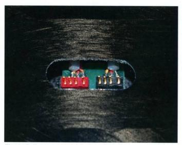
Flap and aileron connectors are pre-installed
