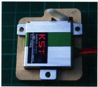
KST 135 flap servo has hefty side mounting lugs for direct fixing to the ply frame. Metal gears seem very durable and the servo yields easily if the controls are touched when handling, which is an important feature to save damage
