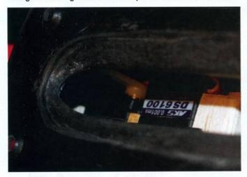
Servos in place. There's not much room but being quickly removable makes things easier and allows the receiver to be positioned behind them
