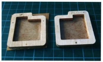
Servo trays backed with thin ply before and after trimming. This allows positioning and installing without the fear of also gluing the servo permanently in place! Remember to clear the glue from the screw holes
