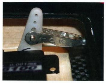
Since the geometry of the linkages required such a short servo horn, one side of the metal link needed a little relief to avoid binding
