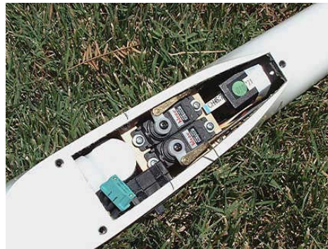
Servo Installation – Electric Fuselage. If larger batteries are used then the elevator servos may have to be fitted behind wing T/E.
