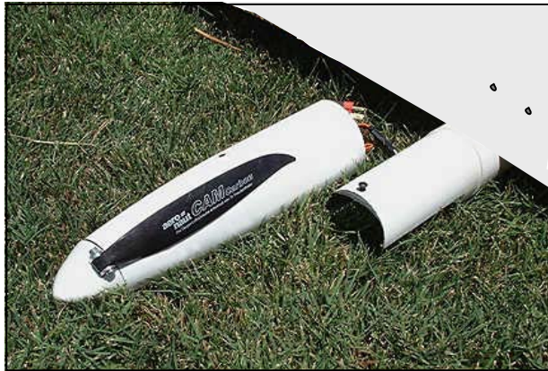
Electric fuselage with Nose cone removed, showing prop and spinner
