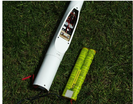
Electric fuselage with Nose cone removed 10 x 1250 cells shown
