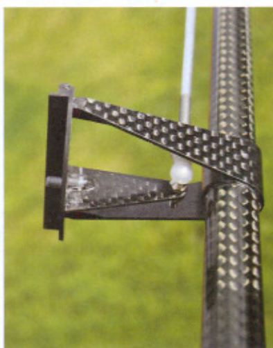
An all-moving tailplane avoids incidence issues, but it needs to be well supported. Here, then, the Hyper Ava uses Vladimir's models favoured V mount to good effect.
