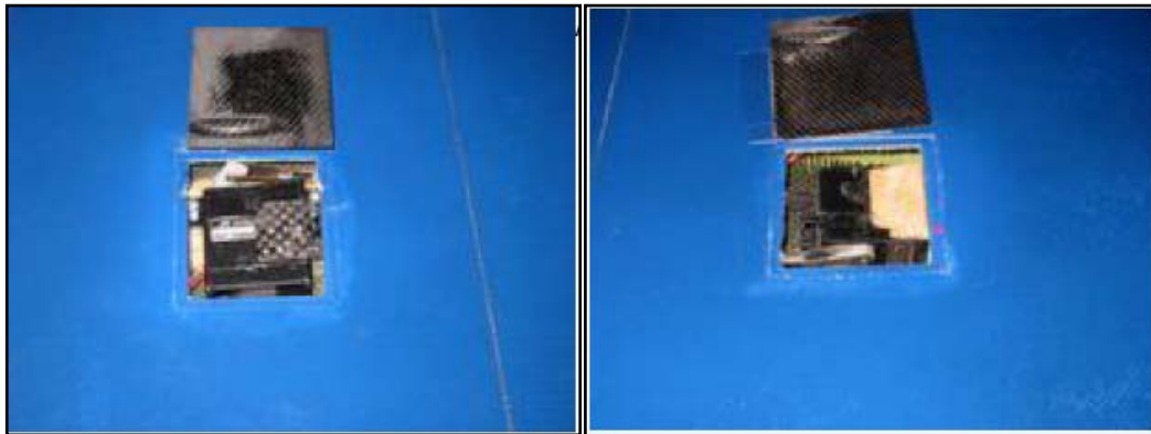
Pic.14 – Servos connected to the upper wing skin
