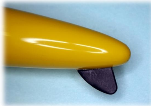
Installed Landing Skeg
