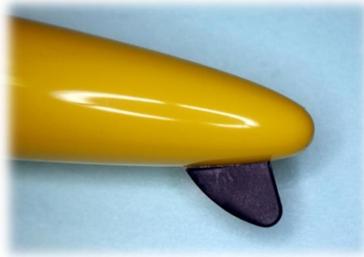
Figure 7: Installed Landing Skeg
