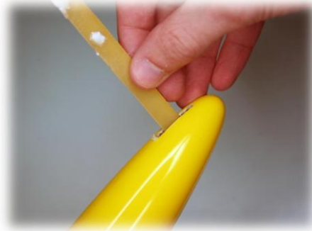
Figure 5: Adjusting the mounting bracket through the slot cut in the fuselage
